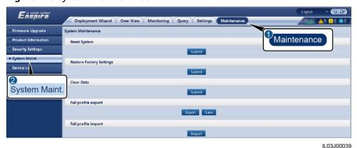
FunctionDescriptionReset SystemResets the SmartLogger, which will automatically shut down and restart.
