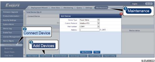
ParameterDescriptionDevice TypeSet this parameter to Power Meter.Comm. ProtocolSet this parameter to Modbus-RTU.Port numberSet this parameter to the serial number of the COM port connected to the power meter.AddressSet this parameter to the communication address of the power meter.
