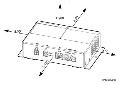
Figure 3-2 Recommended installation space (unit: mm)
