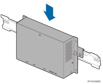
**Step 3** Use two M4x8 screw assemblies to secure support 2 to support 1 to a torque of  $1.2 \text{ N} \cdot \text{m}$ , as shown in Figure 3-7.
