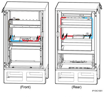
Figure 4-3 Cable routes (SUN2000 communication box scenario)
