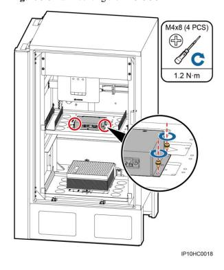
Figure 3-3 Ear-mounting the PLC CCO
