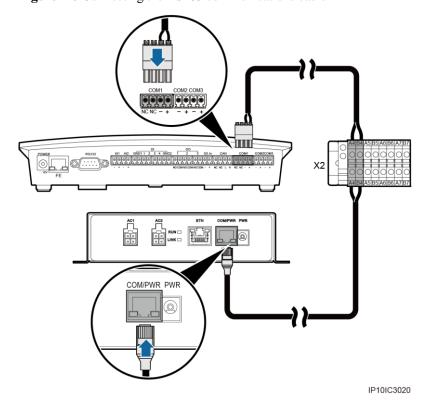
Figure 4-6 Connecting the RS485 communications cable
