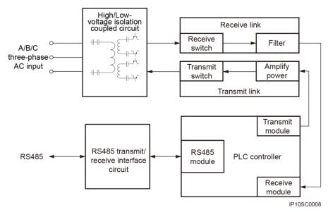
The working principles of the PLC CCO are as follows:
