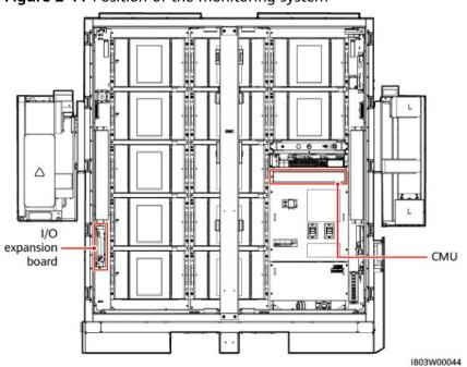
Figure 2-11 Position of the monitoring system
