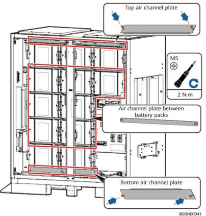
Figure 7-21 Installing air channel plates
