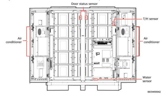
Figure 2-13 Position of the environment control system
