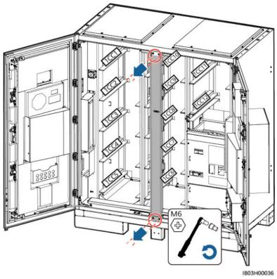
Figure 7-13 Removing the column
