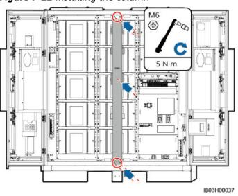
Figure 7-22 Installing the column
