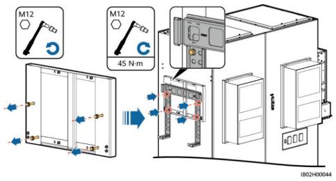
Figure 7-29 Installing a mounting bracket
