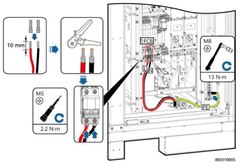
Figure 8-11 Connecting AC Power Cables
