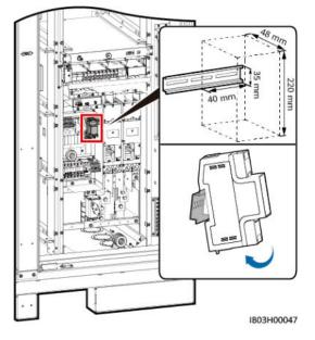
Figure 7-33 Installing the DDSU666-H
