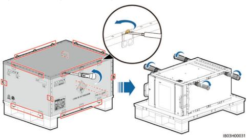
**Figure 7-17** Taking out the battery pack
