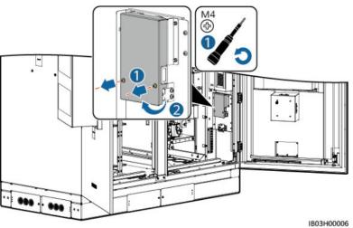
Figure 8-15 Removing external mechanical parts
