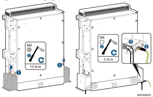
Figure 8-9 Connecting a ground cable
