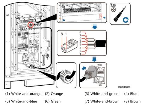
Figure 8-13 Connecting a FE communications cable
