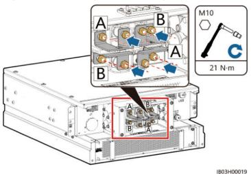
Figure 7-24 Installing short-circuiting copper bars
