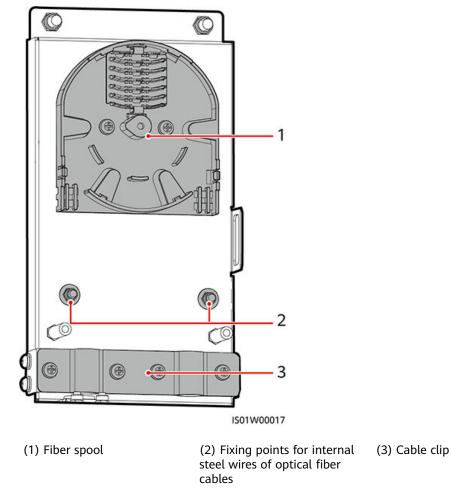
Figure 8-14 Access terminal box (ATB) interior
