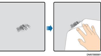
**Step 2** Dip a piece of cotton cloth into anhydrous alcohol and wipe the polished or damaged area to remove dirt or dust. Then wipe off the alcohol with a clean and dry cotton cloth.
