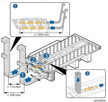
Figure 7-16 Assembling the installation kit
