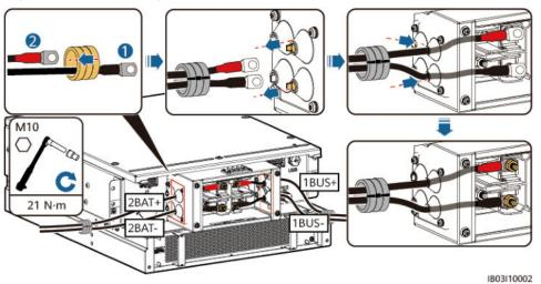
Figure 8-6 Connecting cables
