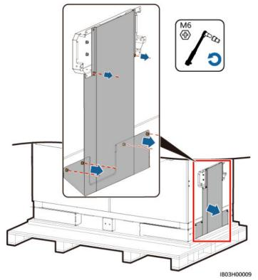
Figure 7-1 Removing the bottom baffle
