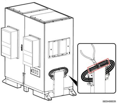
Figure 7-26 Removing bound cables
