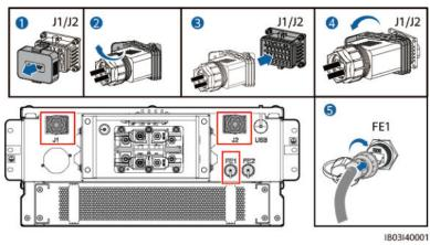
Figure 8-7 Connecting cables
