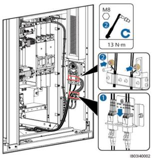
Figure 8-17 Connecting optical fiber cables
