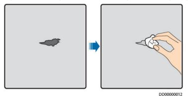
**Step 3** Paint zinc-rich primer on the damaged coat.
