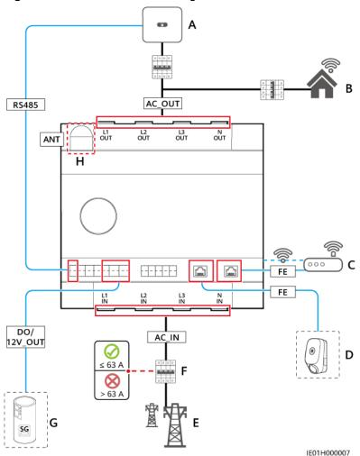
**Figure 5-1** Cable connection diagram: internal CT connection (current ≤ 63 A)
