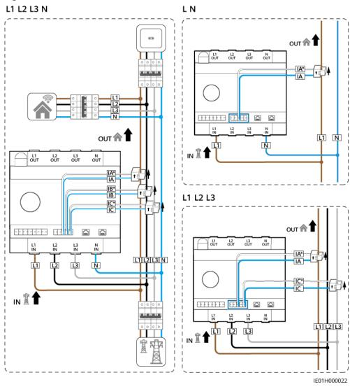
Figure 5-8 External CT connection (current > 63 A)
