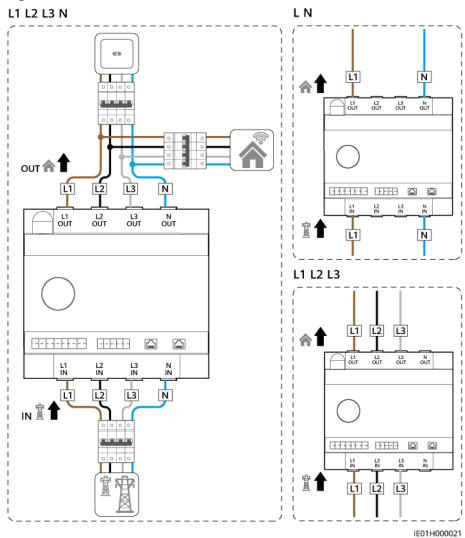
Figure 5-7 Internal CT connection (current ≤ 63 A)
