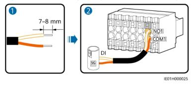
**Step 3** Insert the 14-pin signal connector into the EMMA.
