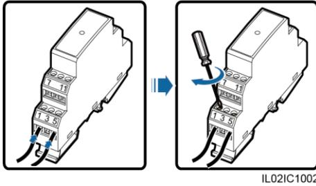
5. Connect the other end of the cable to the communications port on the device.
