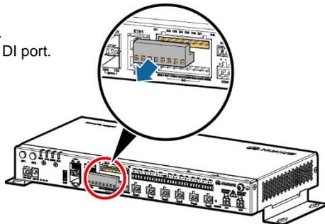
4. Connect the stripped cable core to the terminal block of the DI port on the SmartLogger.
