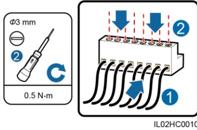
5. Insert the terminal block into the SmartLogger DI port.
