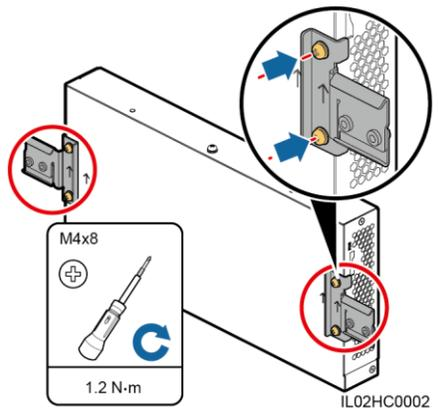
3. Mount the SmartLogger onto the guide rail.
