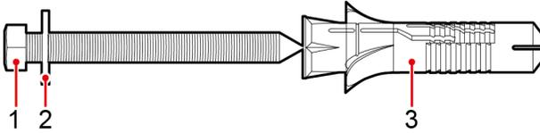
Screw assembly for wall-mounting:
