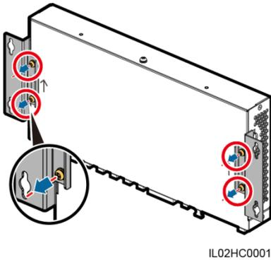
2. Secure the guide rail clamps using the screws that are removed from the mounting ears.
