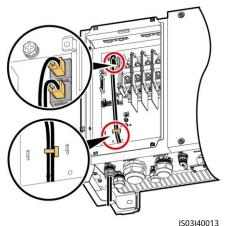
7. Use a torque wrench with an open end of 33 mm to tighten the locking cap to a torque of 7.5 N·m, and seal the waterproof connector.
