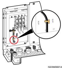
7. Use a torque wrench with an open end of 33 mm to tighten the locking cap to a torque of 7.5 N·m, and seal the waterproof connector.
