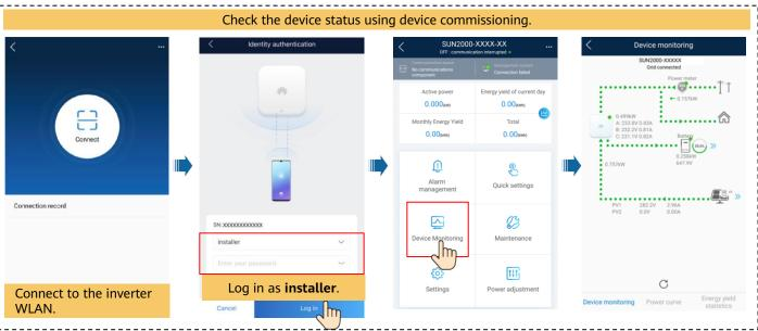
• Checking the Device Status Remotely.
